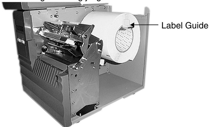
4. Feed the labels under the label guide shaft, through the print head assembly and out of the front of the printer.
