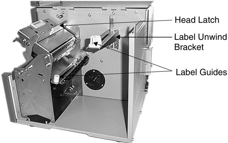
3. Load the media roll onto the label unwind bracket so that the printing side of the labels faces upwards as it unwinds from the roll. Push the roll all the way to the inside of the printer and the label unwind guide snugly against the outside of the label roll.
