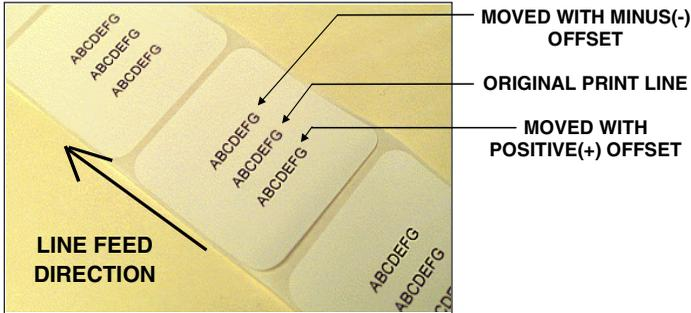
The label pitch is the distance from the leading edge (the edge that comes out of the printer first) of a label and the leading edge of the next.
