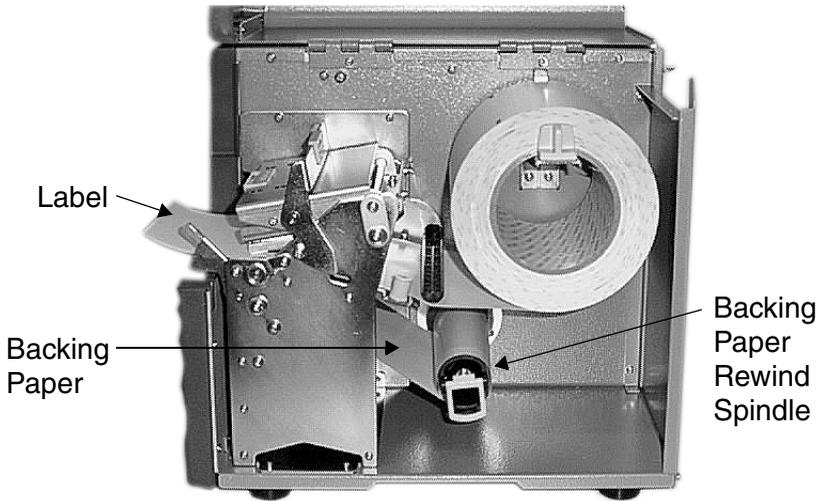
5. Inspect the label route and check that the path matches that illustrated in the label loading diagram. Set the adjustable label guides to keep the labels against the backplate of the printer. Close the print head assembly by pushing down the the green button.
