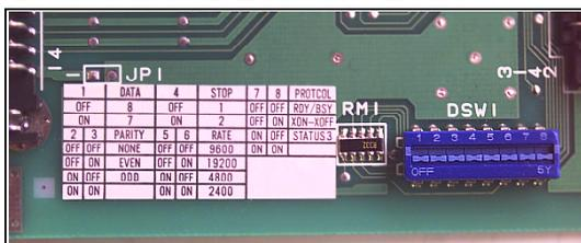
To set the switches, first power the unit Off, then position the DIP switches. After placing the switches in the desired positions, power the printer back on. The switch settings are read by the printer electronics during the power up sequence. They will not become effective until the power is cycled.
